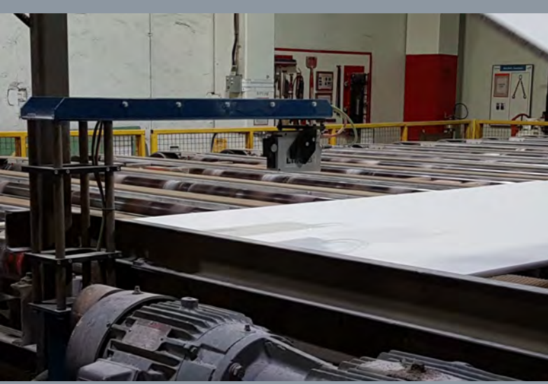
Thickness profile measurement
